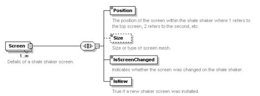
Each instance of the Screen element contains all the details of a shale shaker screen. The standard does not enforce any specific ordering to the instances of these elements but they should be in the order of top screen first, then the middle screen and then the bottom screen.
