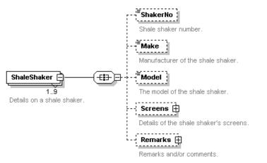
Each instance of the ShaleShaker element contains all the details of a shale shaker. The standard does not enforce any specific ordering to the instances of these elements but they would typically be in the order in which they were recorded.
