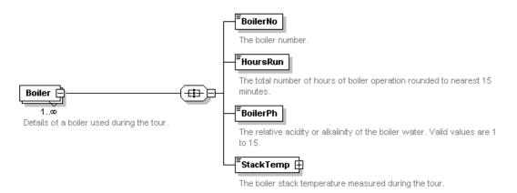
Each instance of the Boiler element contains all the details of a boiler used during the tour. The standard does not enforce any specific ordering to the instances of these elements but they would typically be in the order in which they were recorded.
