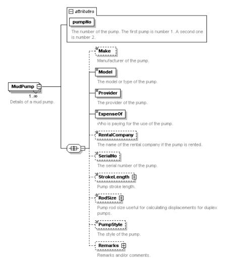
Each instance of the MudPump element contains all the details of a specific mud pump. The standard does not enforce any specific ordering to the instances of these elements but they would typically be in the order in which they were recorded.
