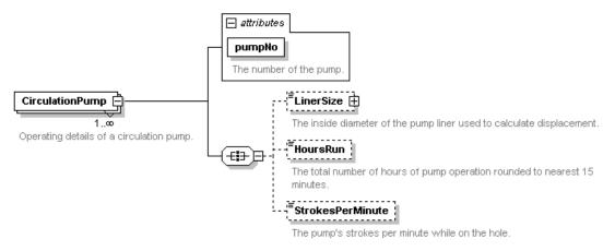
Each instance of the CirculationPump element contains the operating details of a circulation pump. There is no particular order to the instances of this element but each instance corresponds to a specific pump and, as such, each must have a unique value of pumpNo.
