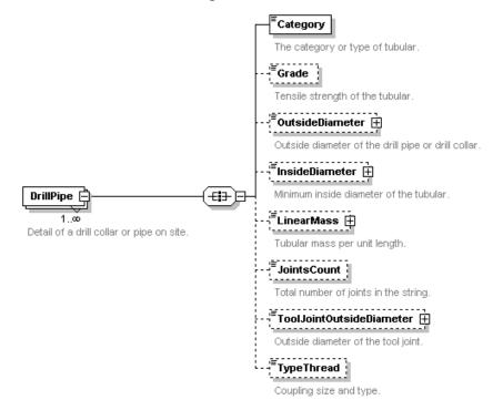
Each instance of the DrillPipe element contains all the details of a specific type of drill collar or pipe. The standard does not enforce any specific ordering to the instances of these elements but they would typically be in the order in which they were recorded.
