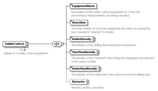
Each instance of the SolidsControl element contains all the details of a solids control equipment. The standard does not enforce any specific ordering to the instances of these elements but they would typically be in the order in which they were recorded.
